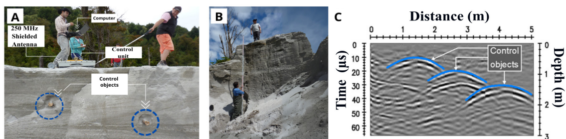
FIG. 4. A. GPR operating along the edge of the gully, woody logs were installed into the steep bank of the gully as control objects (circles). B. Field photograph of the gully where the measures were carried out (about 3.6 m-high). C. Radargram obtained from profile shown on A.
