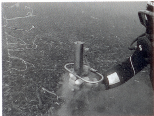
FIG. 2. Current meter employed to determine wind and underwater current directions and device used to sample bottom sediments.
