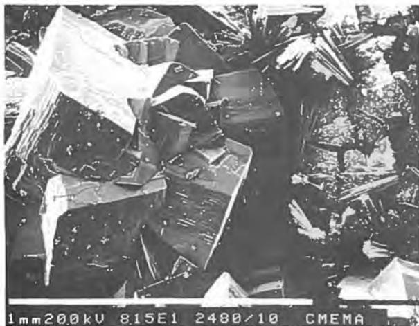
FIG. 8. SEM photomicrograph showing well-formed rhombohedral chabazite crystals (sample 2364).
